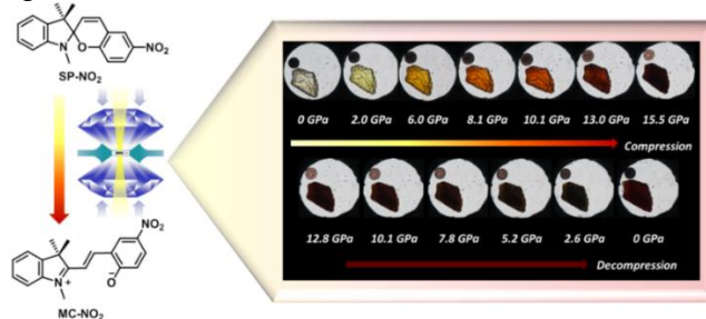
Figure 1. Schematic representation of visible mechanochromic responses of spiropyran in crystal via pressure-induced isomerization.
